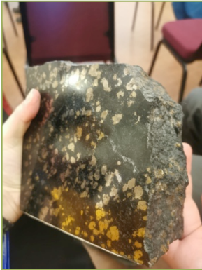
Figure 2: Sample of a polished ultramafic host rock containing PGM, as brought in by Dr Rimmer.
