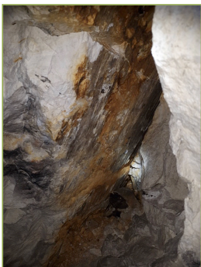
Figure 5: Slickensides observed on the left chalk block.
